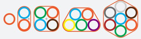
Höhle microducts are designed for long term protection of fiber optical cables. Direct Install (DI) type of microducts are thin-walled products designed to be installed into a conduit that provides the primary mechanical protection for innerduct and cable pathway.
